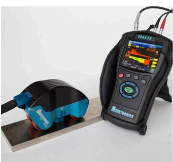
ECHO series in split screen A and B-Scan with optional EZ-Scan 6 magnetic wheel encoder
