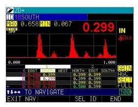
ECHO 9DL – Includes Datalogger, B-scan, Temperature Correction. Gridview A-scan shown above.
