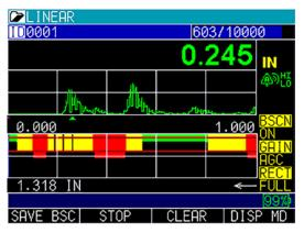
ECHO 9DLW – Includes Waveform, Datalogger, B-scan, Coating Thickness, Temperature Correction, Rubber Boot
