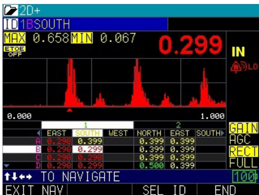
ECHO 9DL – Includes Datalogger, B-scan, Temperature Correction. Gridview A-scan shown above.
