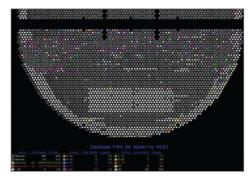
Zetec's Velocity/DM is inspection management software for organizing, tracking, and creating reports of eddy current inspection.
