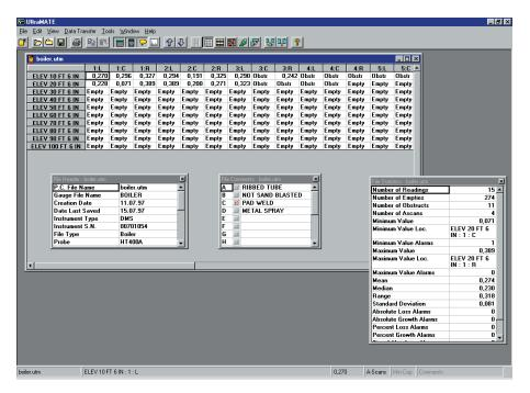
**UltraMATE** is an easy-to-use program for the management of thickness measurement data. It ensures transfer, storage, analysis and documentation of the data, and it makes extensive user-friendly functions available - for example for professional test report layouts.
