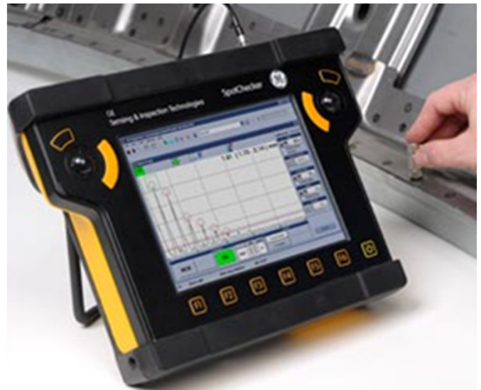
Figure 1: Spot weld inspection with the SpotChecker
