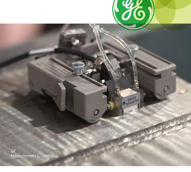
Weld inspections are crucial during the manufacturing process, as well as on a regular basis to ensure weld integrity. Inspections with conventional ultrasonic angle beam probes are time consuming and provide limited
