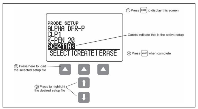
FIGURE 3-2—Selecting a Setup File
