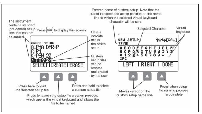
FIGURE 3-5—Follow this procedure to create or erase a Custom Setup file. Custom Setup file names may contain up to 16 characters.
