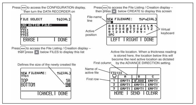
FIGURE 2-4—FILE DISPLAY MODE – When installed and activated, the data recorder option allows users to create data recorder files, store thickness readings (and accompanying A-Scans), and navigate through file contents as shown here. See Chapter 5 to work with Data Recorder files.
