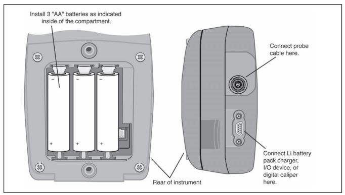
FIGURE 1-1—Insert batteries as shown here. Notice the location of the External Power Connector to which the instrument's Li battery pack's charger be connected.
