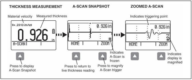
FIGURE 4-1—NORMAL view mode displays only the thickness reading. Selecting the A-SCAN function bar option allows you to view a Snapshot of the A-Scan echo that is represented by the thickness reading. This A-Scan is frozen. No live A-Scan echo is available in this view mode.
