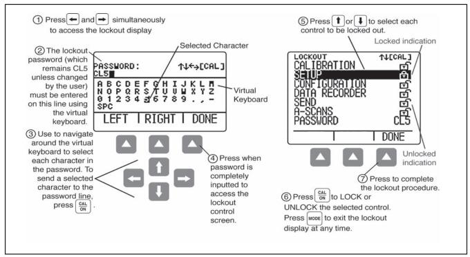
FIGURE 3-6—Procedure for locking and unlocking function keys
