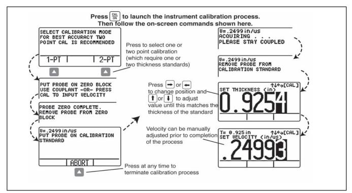
FIGURE 3-4—Instrument Calibration Procedure
