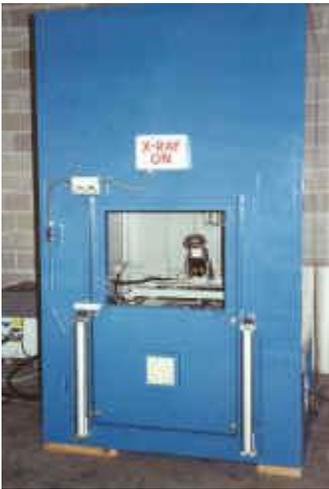
320kV real-time cabinet with pneumatic part door, four axis manipulator, and motorized (adjustable FFD), tubehead elevator.
