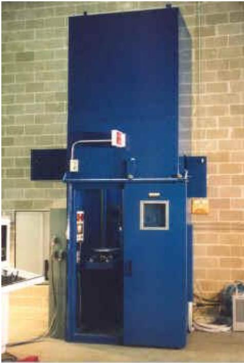
This 225kV real-time x-ray cabinet was custom designed for vertical scanning of parts up to 72" in length while minimizing the use of valuable floor space.
