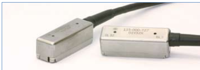
Wide Coverage Corrosion Array - (GEIT Global PN 1314599) • 5 Mhz, 48 mm (1.890") active length with selectable 3 or 5 element apertures • 28 or 30 virtual probes covering up to 44 mm (1.73") • Benefits: Wide coverage with great near surface resolution and flat acoustic response
