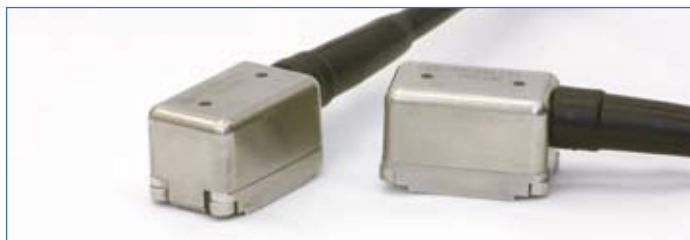
Medium Coverage Corrosion Array (GEIT Global PN 1314600) • 5 Mhz, 24 mm (0.945") active length with selectable 6 or 10 element apertures • 23 or 27 virtual probes covering up to 20mm (0.79") • Benefits: Medium coverage with great near surface resolution and very flat acoustic response • Small footprint improves coupling on curved surfaces and increases lateral resolution
